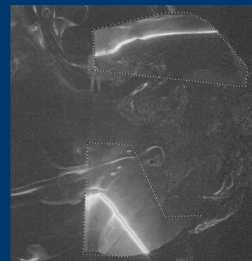
Figure 3: PIV capture of flow field around FWMAV
