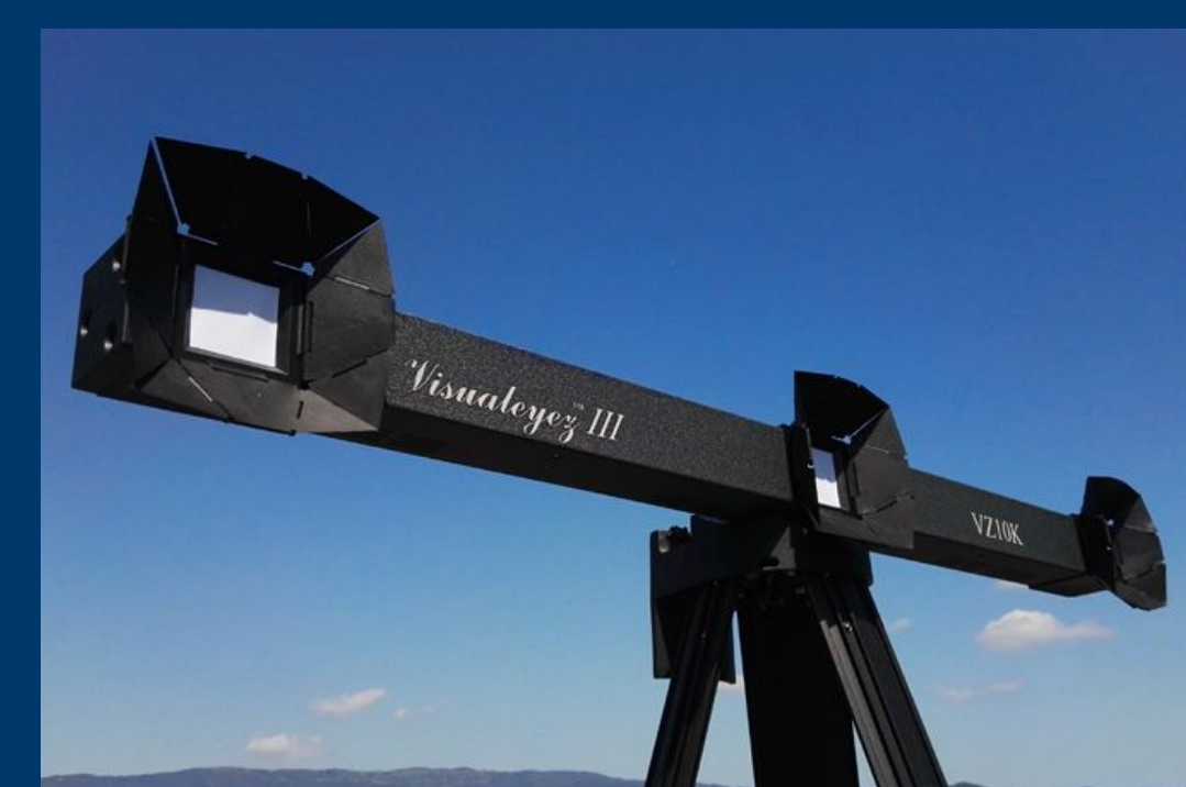
Figure 5: 3D Motion Capture Camera by PTI Phoenix Technologies
