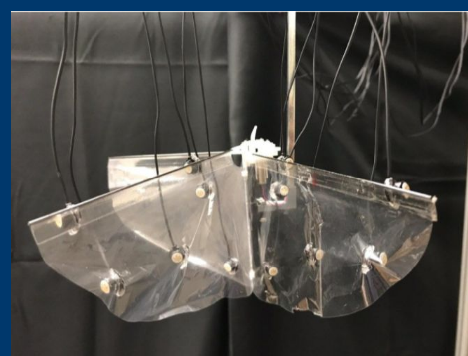
Figure 4: 3D Motion Capture LED trackers on the wings
