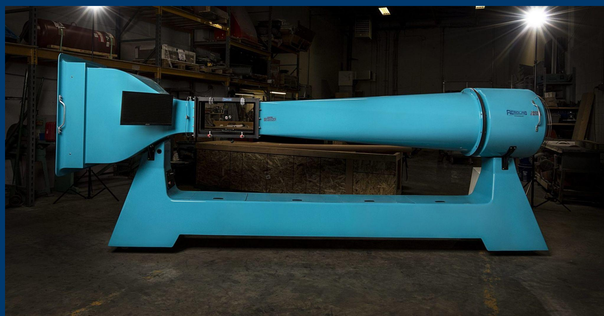
Figure 1: Low Speed Wind Tunnel (Credit: Aerolab)
