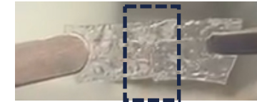
Self-healing of a damaged ICM
