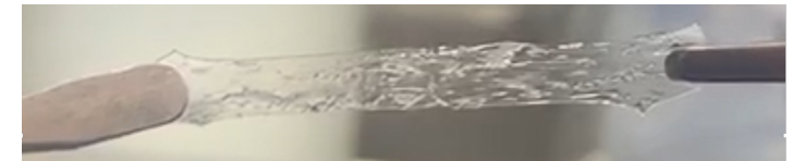
Self-healing of a damaged ICM
